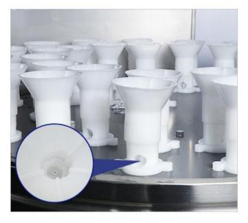
Bottle holder is designed for holding and fixing bottles during washing, it is possible to customize bottle holders according to different sizes of bottles Make sure the machine can work perfectly. There is a filling nozzle in the bottle holder which is designed for cleaning the inside of bottles.
