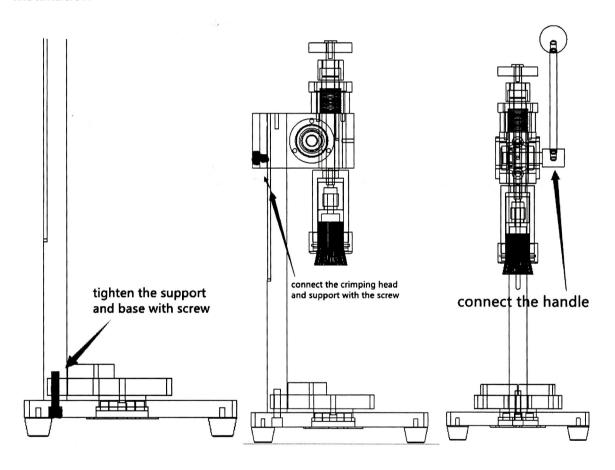
At the first time to use, please hold the top and press the hand handle several times, to let the machine run smoothly
