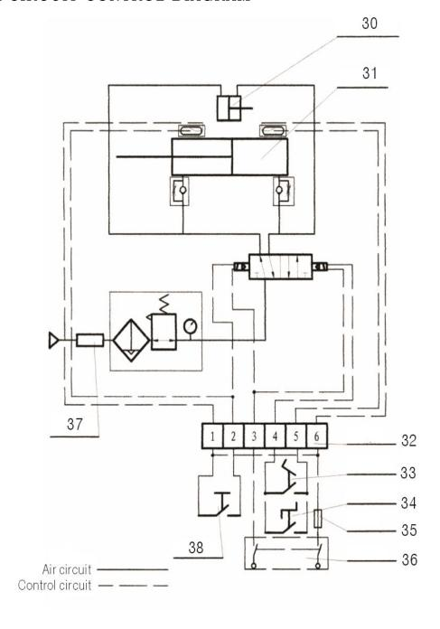
30. Cylinder for material filling nozzle 31. Cylinder for material pushing
